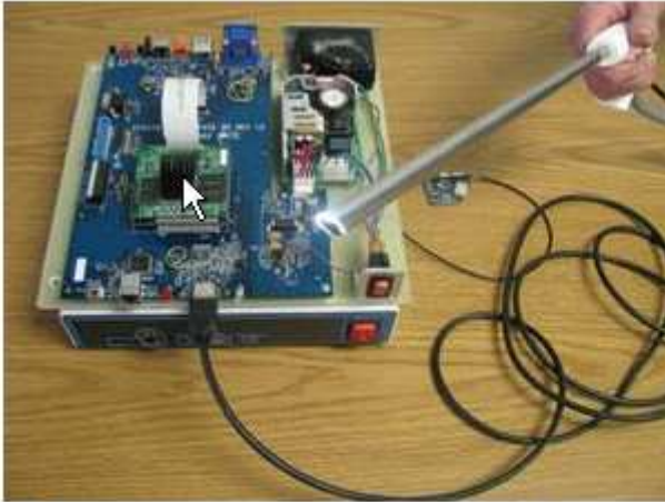
FIGURE 2. After images are transferred over 2 m of HDMI cable, they are processed by an embedded computer. This consists of a baseboard that allows the unit to output a variety of video formats such as VGA, NTSC, Ethernet, and S-Video, a stack of three boards used for I/O, CPU control, and an FPGA board that processes image data in real time.
