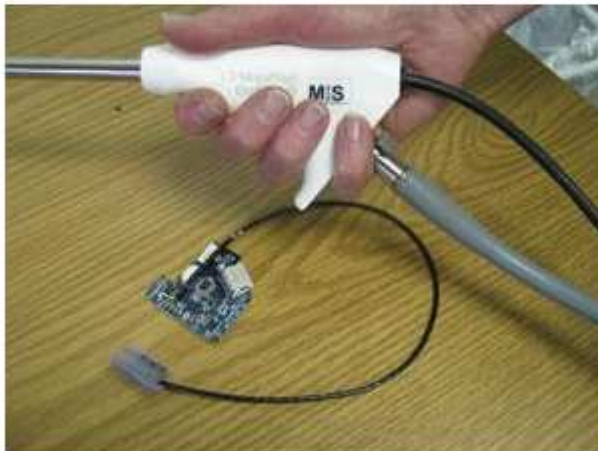
FIGURE 1. In the design of the MIS disposable arthroscope, probe cost was reduced by using a custom CMOS color imager. After 3.3-V analog images are transmitted to the handle, they are amplified, digitized, and transmitted over an HDMI to the unit's controller image data in real time.
